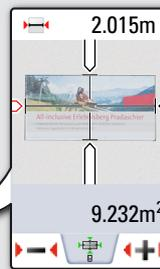
Select arrows with the cursor keys or by tapping on the display and adjust with softkeys. Corresponding area is calculated.
