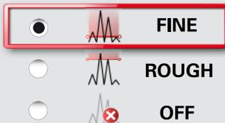
Choose the sensitivity of the levelling, which is needed for some measuring functions. FINE means, that the levelling of the device is sensitive to any small vibrations. Choose ROUGH when working in harsh construction environment with many shocks and vibrations. In this case the accuracy is decreased in correlation with the movements.
