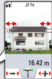
Select arrows with the cursor keys or by tapping on the display and adjust with softkeys. Corresponding width is calculated.
