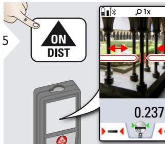
Select arrows with the cursor keys or by tapping on the display and adjust with softkeys. Corresponding diameter is calculated.
